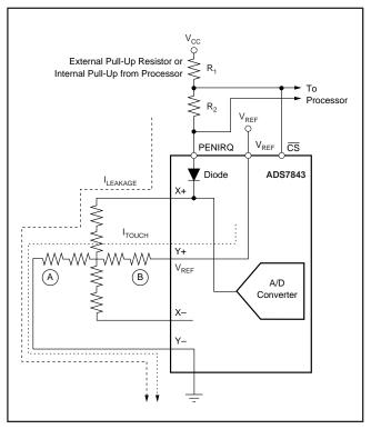
FIGURE 8. Recommended Solution to Minimize Offset Error.
