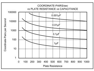
FIGURE 5. Filter Capacitor Selection Depends Upon Plate Resistance and the Number of Coordinate-Pair Readings per Second Desired.
