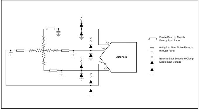
FIGURE 9. Input Protection for ADS7843.
