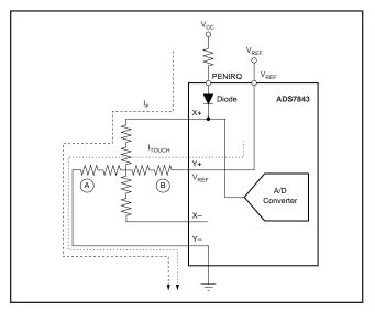
FIGURE 7. Simplified Schematic of ADS7843 for A2A1A0 = 001.
