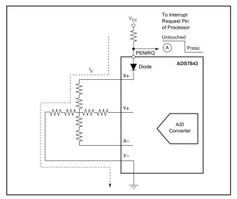
FIGURE 6. Simplified Schematic of ADS7843 for PD0, PD1 = 00.
