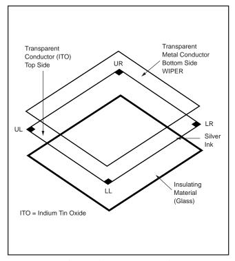
FIGURE 3. 5-Wire Touch Screen Construction.
