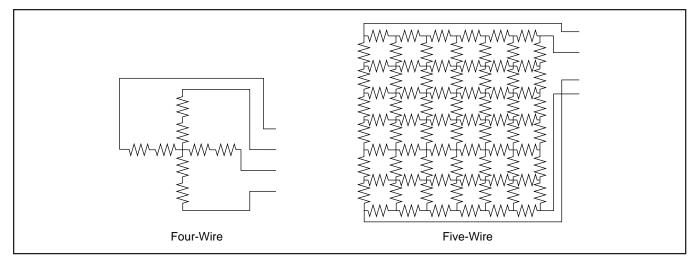
FIGURE 1. 4-Wire and 5-Wire Touch Screen Circuits.
