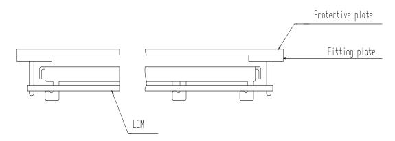
2) When assembling the LCM into other equipment, the spacer to the bit between the LCM and the fitting plate should have enough height to avoid causing stress to the module surface, refer to the individual specifications for measurements. The measurement tolerance should be ±0.1mm.
