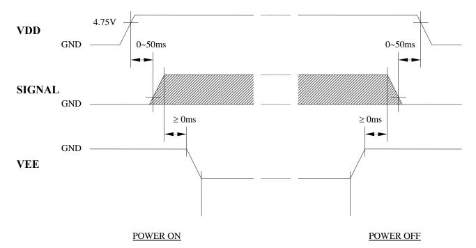
Note: The missing pixels may occur when the LCM is driven except above power supply timing sequence.
