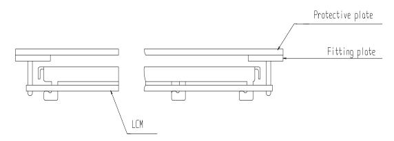
2) When assembling the LCM into other equipment, the spacer to the bit between the LCM and the fitting plate should have enough height to avoid causing stress to the module surface, refer to the individual specifications for measurements. The measurement tolerance should be ±0.1mm.
